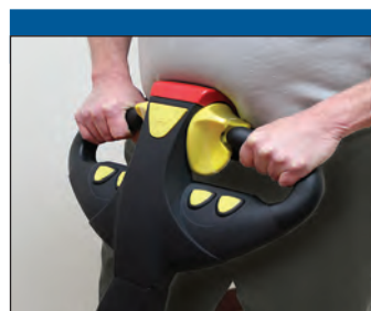
Auto-reversing "belly bump" switch protects against operator accidents while working in tight quarters.
